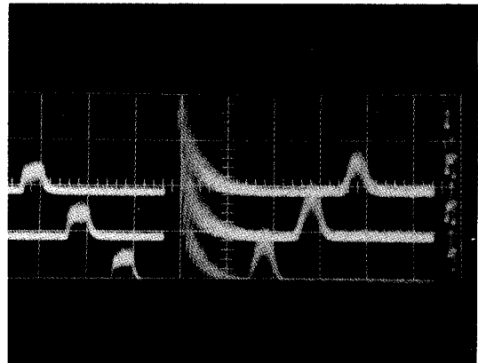
FIG. 6--Multiple exposure shows the time-inverting property of the device after leveling. The time-inverted pulses on the right move in the opposite direction from the input signals shown as leakage on the left. Horizontal scale: 1 \mu s/div.
